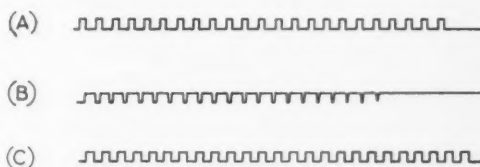
(A) Dot contacts too far apart. (B) Dot contacts too close. (C) Dot contacts correctly adjusted.
